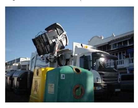
Each communal collection point has been fitted with a heavy duty flood light to help the loading of the Kiggen compactor at night by people, as well as for helping the driver of the hook loader when he collects the container for emptying in the early hours. All communal collection points are also being fitted with CCTV cameras so that the management of FCC can monitor them twenty four hours a day. This is to prevent the theft of one of the Kiggen compactor containers by a rogue waste operator.
