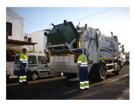
The use of the side loader collection system is more cost efficient as it is quicker compared to the conventional rear loader collection system previously used. It is less labour intensive as it only requires a driver to operate the side loader collection equipment compared to a rear loader which requires a driver and two collection operatives to position the containers at the rear of the collection vehicle for emptying, prior to them be re positioned at the communal collection point.
